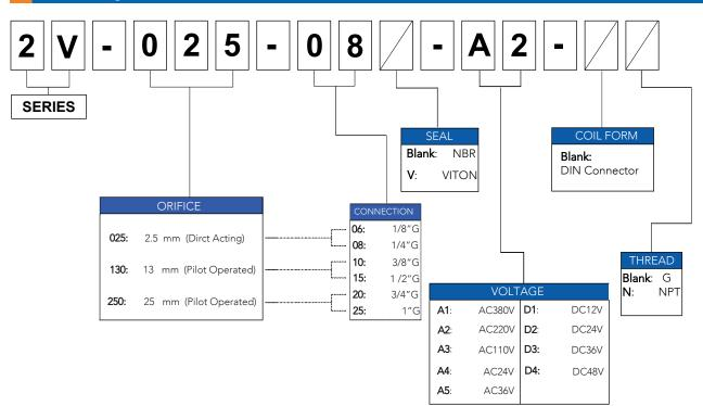
Order Example: 2V series pilot operated 2/2 ways solenoid valve,1/2" port size, VITON seals, AC220V, DIN connector, BSPP (G) thread. SENYA part# 2V130-15V-AC220V
